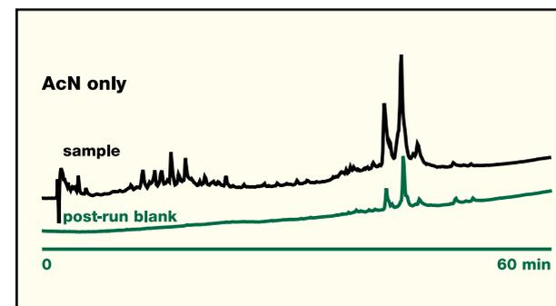
**Figure 4. Examination of post-run blank for chromatogram with acetonitrile only.** Conditions as in Figure 3.
