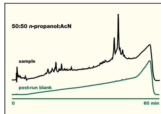
**Figure 5. Examination of post-run blank for chromatogram run with 50:50 acetonitrile:*n*-propanol.** Conditions as in Figure 3.
