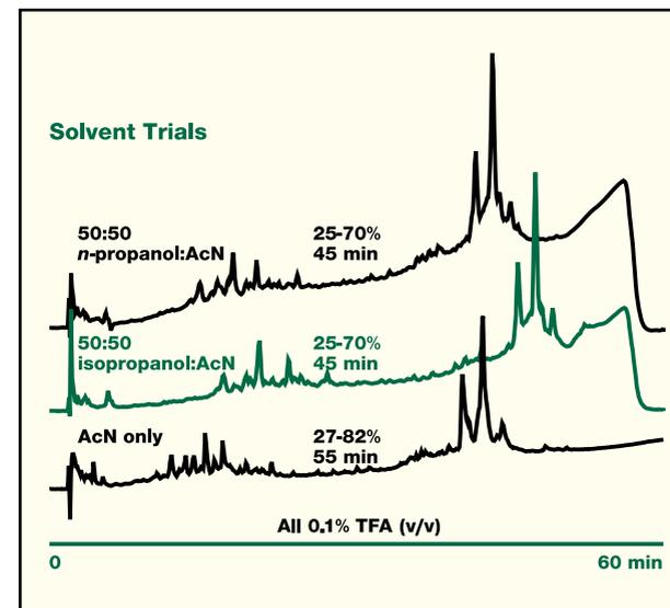
**Figure 3. Trial chromatograms for analytical reversed-phase separation with different eluting solvents.**
